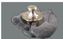
Fig. 3 Weight (200g) Hardness Test (図3 硬度測定分銅(200g荷重))
